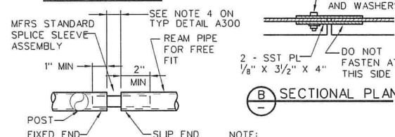
RAIL SLIP JOINT
