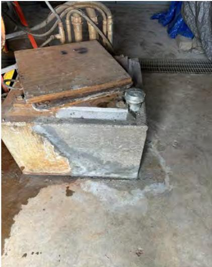
The repaired gravel feed tube and pump stand
