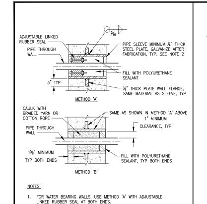
2. SLEEVES ARE NOT REQUIRED IN CORE DRILLED WALLS, PENETRATIONS
