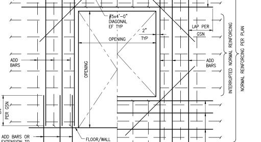
ADDITIONAL REINFORCING AT RECTANGULAR OPENINGS IN WALLS/SLABS
