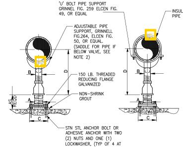
INSULATE METALLIC PIPES FROM PIPE SUPPORT
