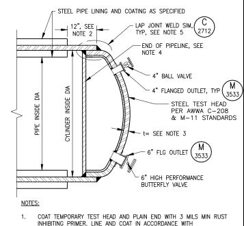
FOR STATION AND LOCATION OF PIPELINE ENDS, SEE DRAWINGS.
