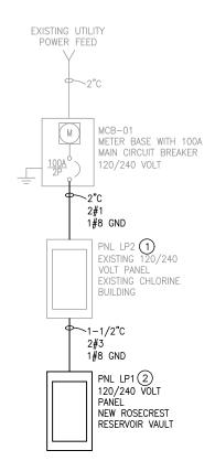
MODIFIED POWER ONE—LINE DIAGRAM SCALE: NTS
