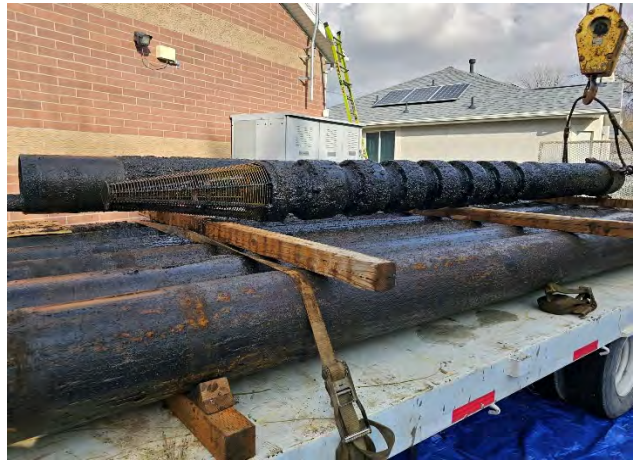
Existing pump and column pipe
