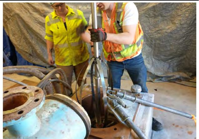
Pulling the scanner out of the well
